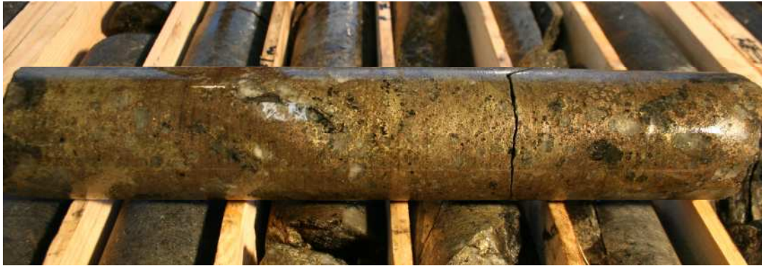
Photograph 1: High grade copper mineralisation from 70.4 to 70.8 m in Hole 12-09 containing chalcopyrite-pyrite-pyrrhotite. This mineralisation makes up part of a 6.35 m intersection (68.80 to 75.15 m) containing 2.38 % Cu and 2.85 g/t Au.
