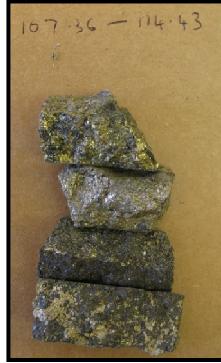
Drill hole BH D 107.36 to 114.43 Massive pyrite and chalcopyrite sulphides with magnetite matrix.
