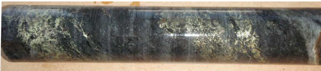
Sulphide intersection, Hole 17-10, 173m
