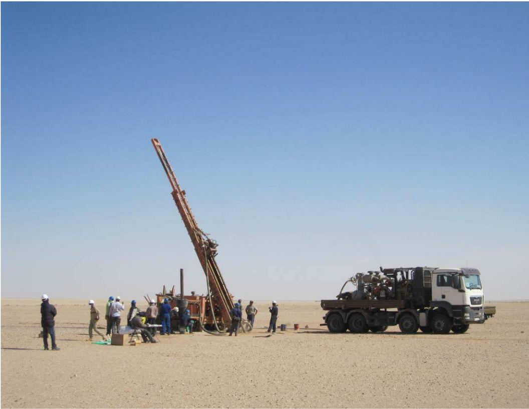
*Figure 2: RC rig on site at Conchita, January 2012*
