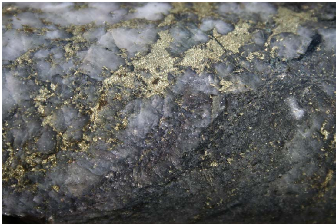
Hole 21-10, 17.5m depth: pyrite and bismuth minerals in gold-copper ores
