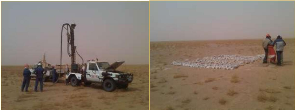
*Fig. 2: Air core drilling & collection of samples at Tasiast South Project, Mauritania*
