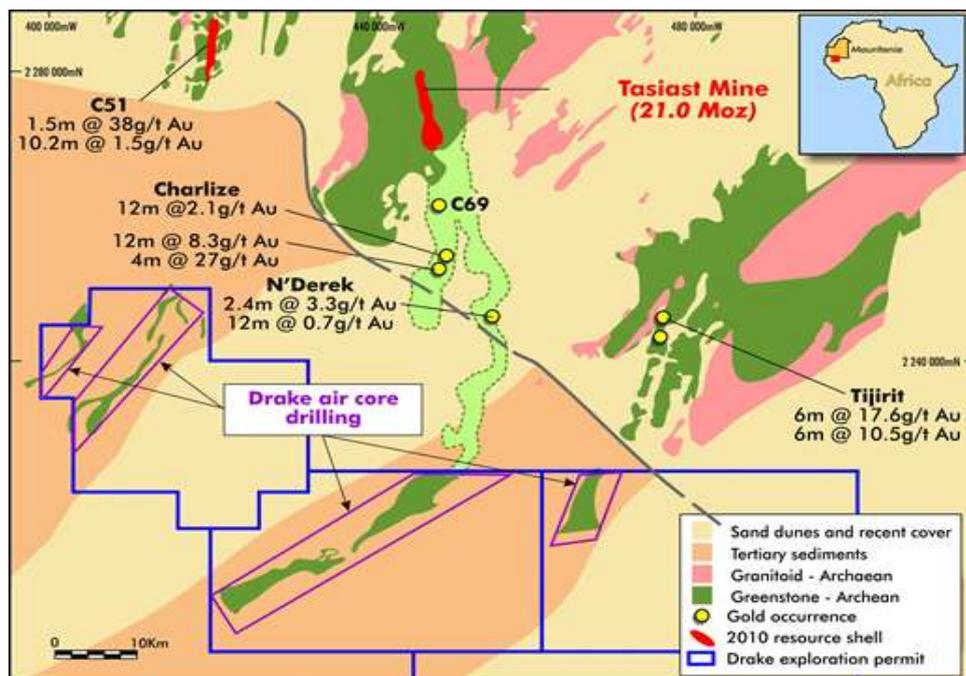
Fig. 1: Greenstone belt extensions under cover within Drake's Tasiast South Project Area
