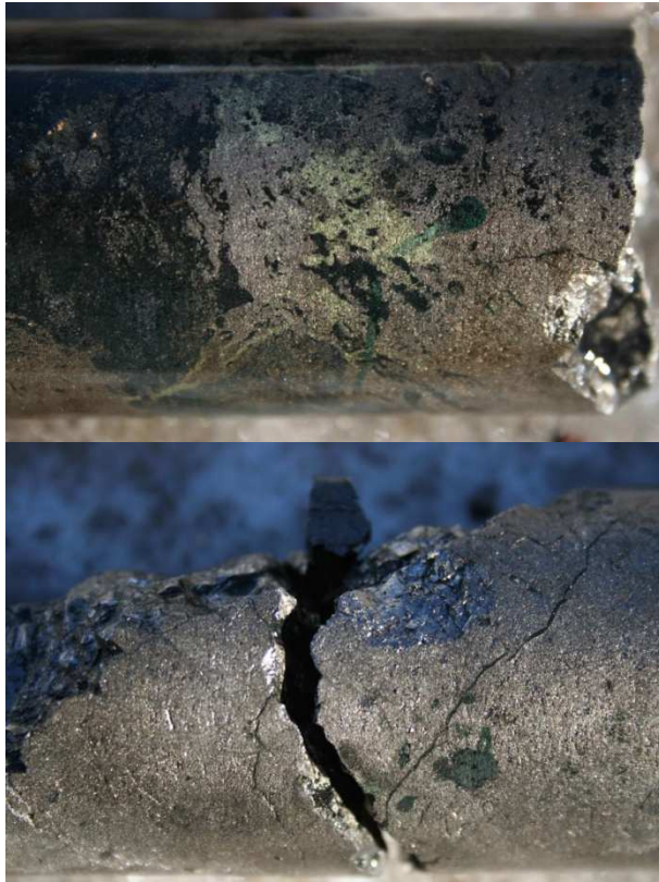
Figure 2: Left – Approx 184 m, semi massive pyrrhotite and chalcopyrite; Right – Approx 217m, massive pyrite mineralisation. Core size is NQ.
